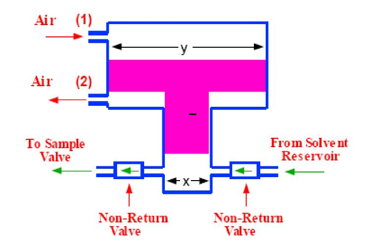
Figure 4. A Diagram of the Pneumatic Pump
