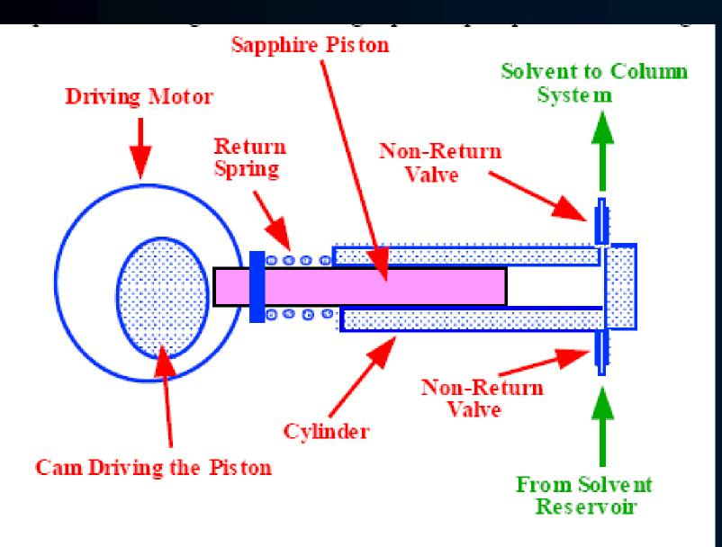
Figure 7. A Single Piston Reciprocating Pump
